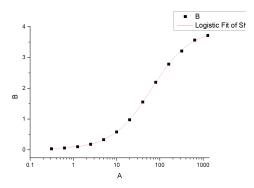
Four-parameter fitting standard curve (linear correlation coefficient R2=0.9999)
